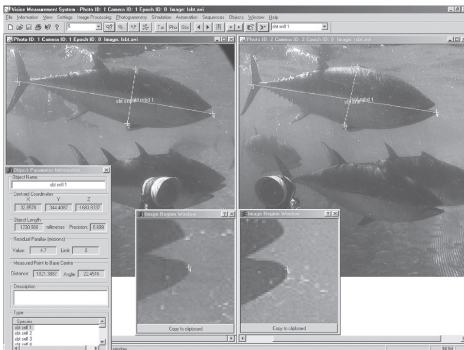
Fig. 7. Screenshot of a bluefin tuna being measured in the EventMeasure program for stereo-DOV video analysis from a previous study. (Photograph adapted from Shortis et al., 2009).
